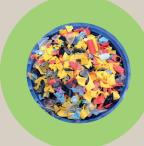
The first step in the recycling process is the granulation of the TipOne® plastic
