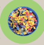
The first step in the recycling process is the crushing of the TipOne® plastic. The shredded material is then processed into plastic granulate
