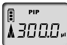
The nominal volume or volume to be tested is set, standard mode Pipetting (PIP), e.g. 200.0 µl (for procedure, see PIP mode). Ex: Volume according to volume test 301.3 µl.
