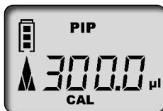
The CAL symbol permanently shown in the display indicates that an adjustment has been made.
