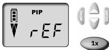
The ErgoOne® E Multi-Channel pipette automatically requests a reference run immediately after the battery is inserted. After pressing the pipetting key, the reference run is carried out, and the instrument is ready for pipetting.
