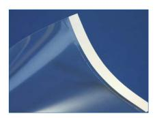
Single coated seal consisting of a 0.05mm polyolefin film coated on one side with a pressure sensitive acrylate adhesive. The seal is supplied on a white paper release liner.
