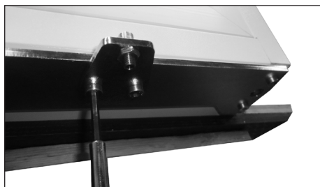
29. Remount bottom handle lockpin plate in the opposite side by tightening the two screws again (use 4 mm allen key)
