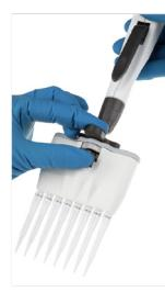
Hold the device over a suitable disposal container and press the ejector to the stop.
