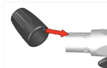
Align mark at the cap when reassembling the cap.
