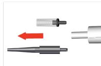
Pull existing adapter with hose out of the hand controller.
