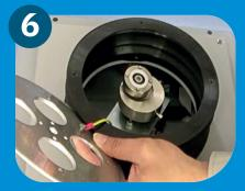
Connect the ground wire with metal flange as in step 3
