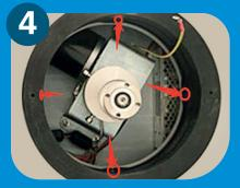
Remove 4 screws which marked with red circle that inside of the rubber locking hose
