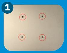
Remove the 4 screws of the shaking plate marked by red circles and keep them well
