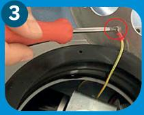
Remove the screw marked by red circle, separate ground wire and metal plate
