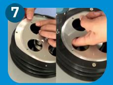
Put the flange into the rubber locking hose and fix it with screws (outer screws as marked in step 2)
