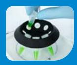
The Tube Rotor holds up to eight microcentrifuge tubes ...
