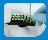
The PCR Strip Rotor holds up to four 0.2 ml 8-tube PCR strips ...
