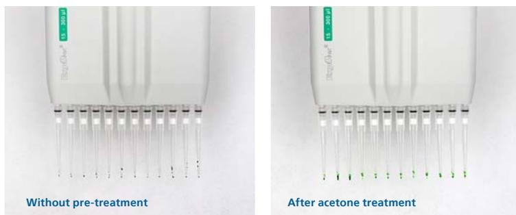
► **Figure 10** Impact on the “Low Retention” effect through acetone treatment on a competitor’s tips.
