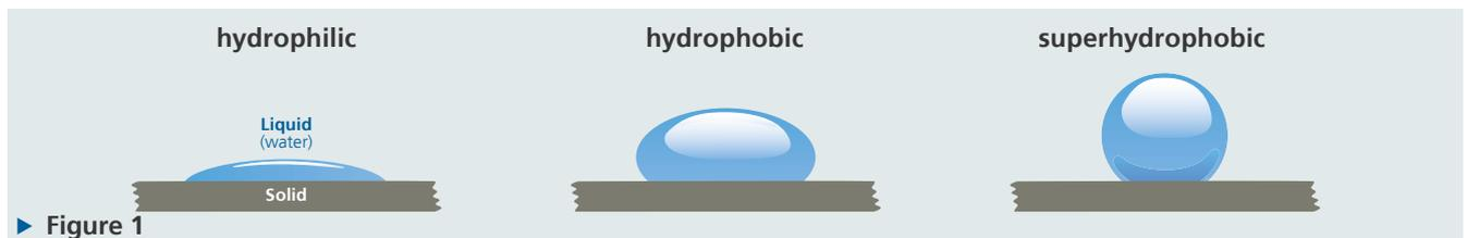
On superhydrophobic surfaces (e.g. the "lotus effect", Fig. 2) water assumes a nearly spherical shape. This means that the contact area between the liquid and the surface is only very small. The droplet cannot stay there and runs off.
