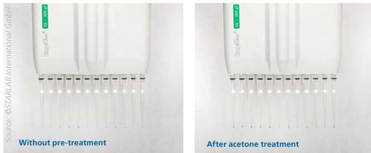
► **Figure 9** Impact on the “Low Retention” effect through acetone treatment for TipOne® RPT tips.
