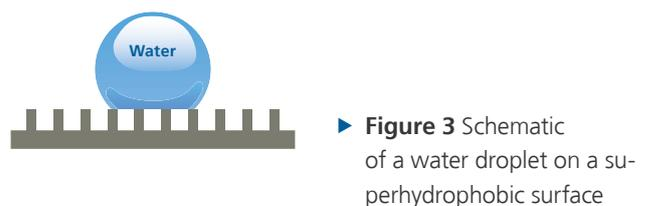
► **Figure 3** Schematic of a water droplet on a superhydrophobic surface
