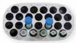
Standard platform (N2400-5104) for 26 tubes up to 15 mm diameter (eg. 1.5 ml, 2.0 ml, 5.0 ml and 15 ml tubes)
